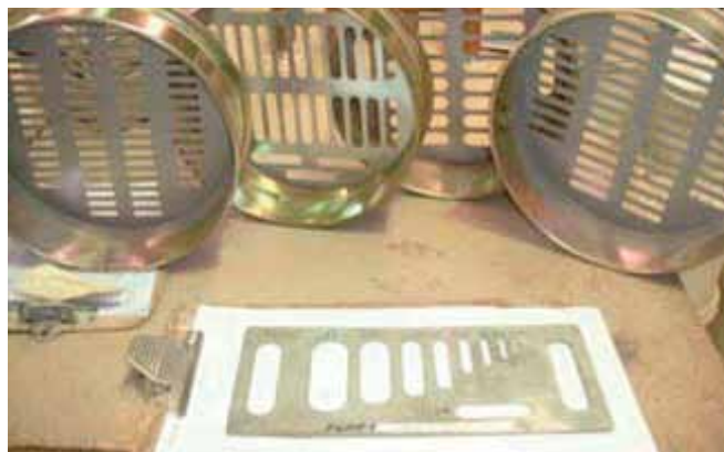
Figure 9: Flakiness Index test gauge and slotted sieves
