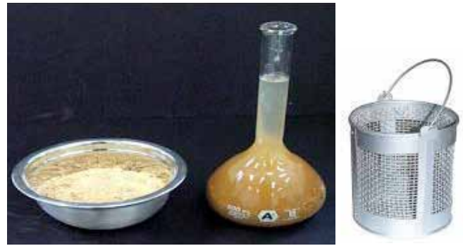
Figure 2: Fine aggregate in a Pycnometer and a wire basket used for coarse aggregate
