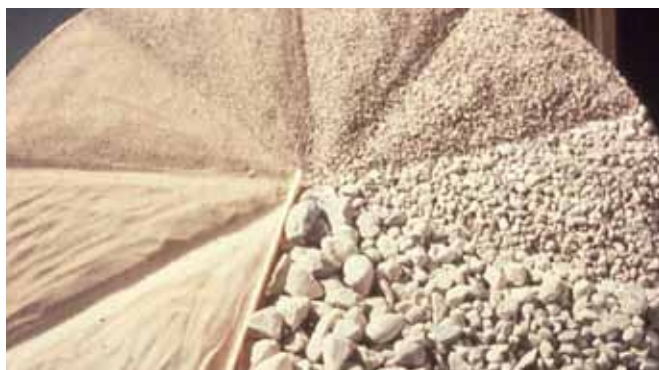
Figure 6: Combined aggregate and sand sample graded into its individual sizes
